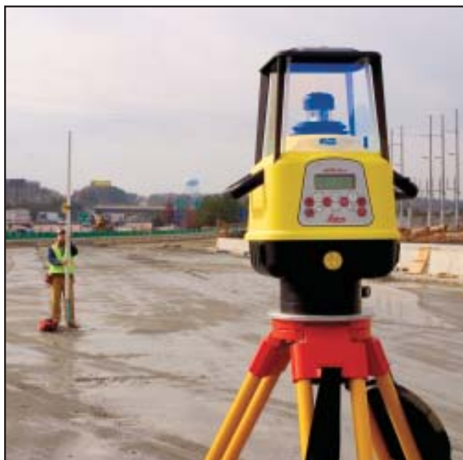
A surveyor shoots an elevation onslope with a Leica Javelin S dual-slope laser on a roadway soon to open.
