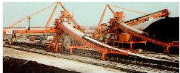
Krupp's bridge-type bucketwheel reclaimer.
