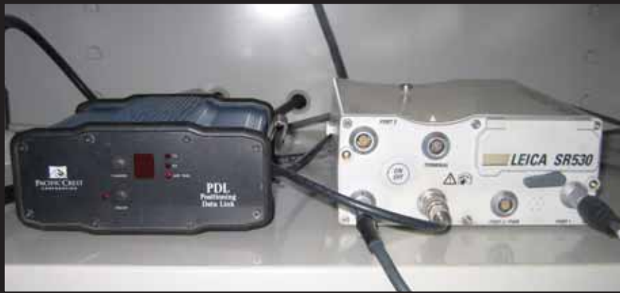
▲ At the base station, a Leica GPS System 500 type SR530 teams with a Pacific Crest PDL HPB radio modem to communicate correction data to the rover
